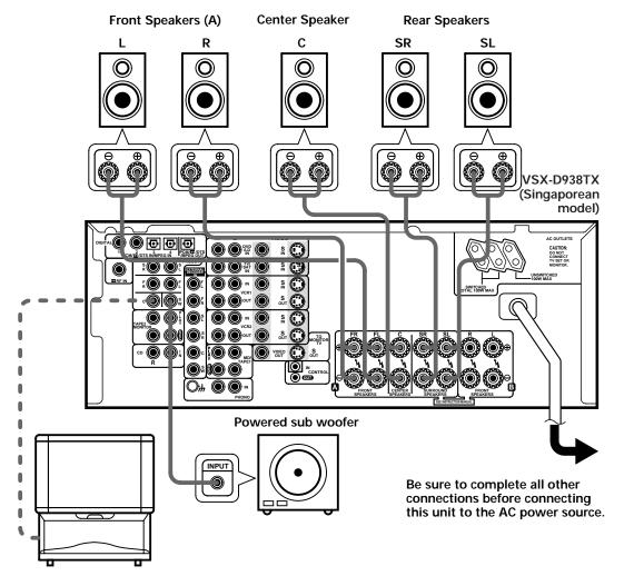
When using the speaker on your TV as the center speaker, connect the CENTER PREOUT jack on this unit to the audio input jack on your TV. In this case, the center speaker shown is unnecessary.
